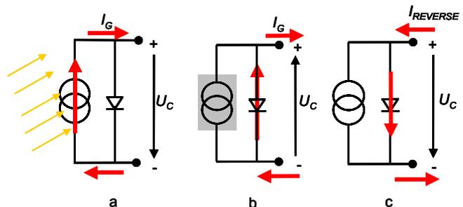
Fig. A7 - Equivalent circuit diagram of a PV cell
