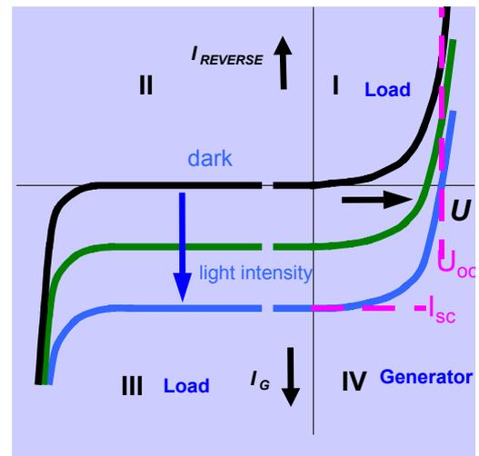
Fig. A1 – PV cell characteristics (Load reference arrow system)
