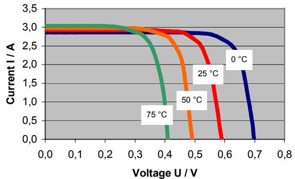
Fig. A3 - Cell characteristics at various temperatures
