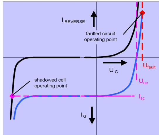
Fig.A9 - Shadowing and fault conditions
