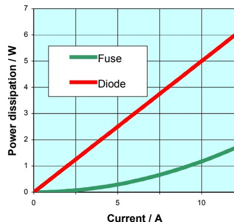
Fig. A13 - Power dissipation of blocking diodes versus PV string fuses
