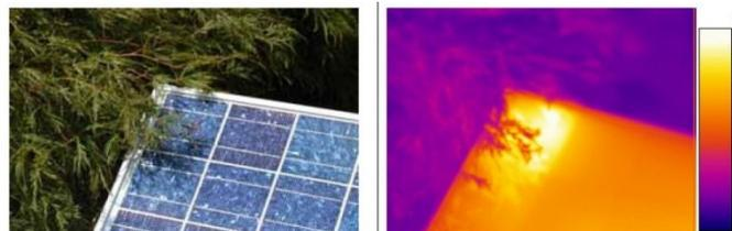
Fig. A8 - Hot spot due to partial shadowing
