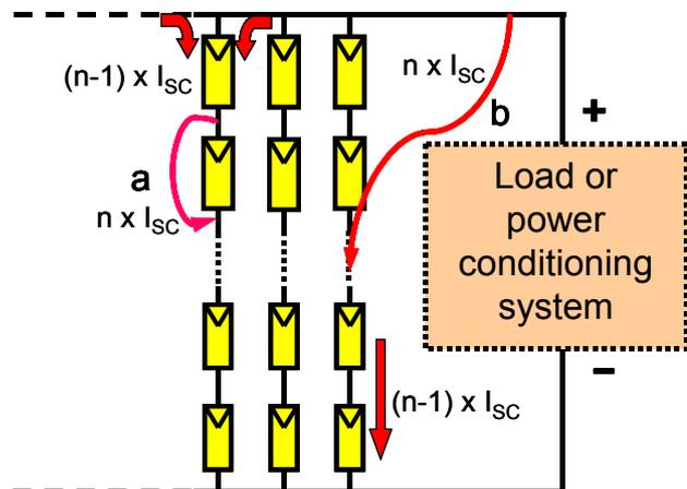
Fig. A10 - Potential faults in a floating PV array
