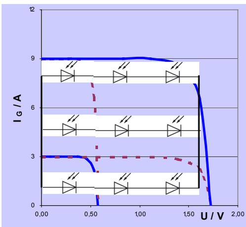
Fig. A2 - Generator characteristics of PV cells connected in parallel and in series
