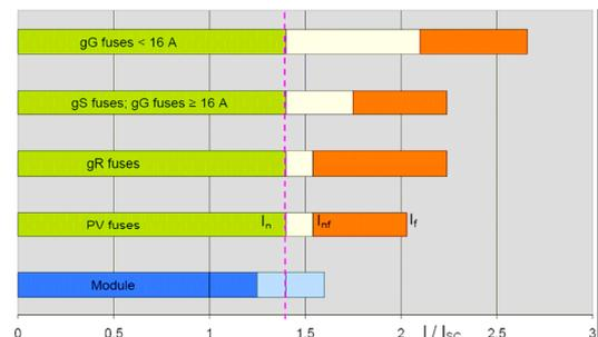
Fig. 2 - Breaking range of different fuse types
