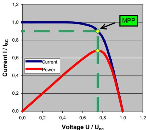
Fig. A4 - Module characteristics
